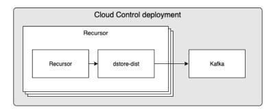
Alternatively, dstore-dist can also be deployed as a standalone set of Pods, to perform additional aggregation, filtering and distribution of protobuf messages sent by multiple sets of DNSdist and/or Recursor pods:
